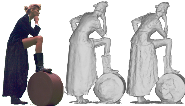
Fig. 1. Challenging scene captured with a passive RGB multi-camera setup [1]. ( left ) one input image, ( center ) reconstructions obtained with classical 2D features [22], ( right ) proposed solution. Our results validate the key improvement of a CNN-learned disparity to MVS for performance capture scenarios. Results particularly improve in noisy, very low contrast and low textured regions such as the arm, the leg or even the black skirt folds, which can be better seen in a brightened version of the picture in Figure 8.
