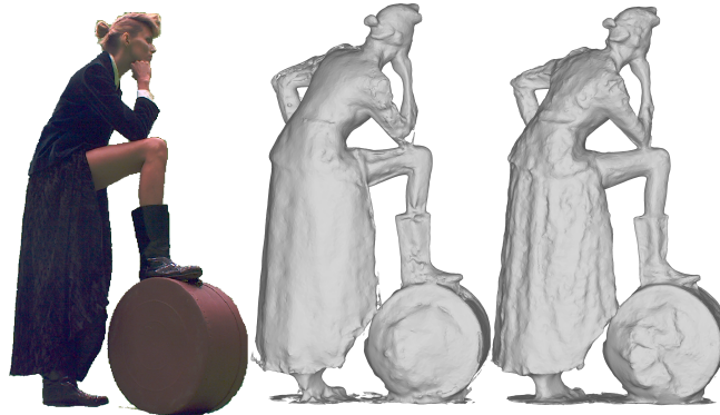
Fig. 1. Challenging scene capture with a passive RGB multi-camera setup [1]. ( left ) one input image, ( center ) reconstructions obtained with classical 2D features [22], ( right ) proposed solution. Our results validate the key improvement of a CNN-learned disparity to MVS for sequence capture scenarios. Results particularly improve in noisy, very low contrast and low textured regions such as the arm, the leg or even the black skirt folds, which can be better seen in a brightened version of the picture in Figure 8.
