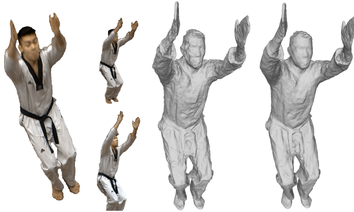
Fig. 9. ( Left ) 3 input images, ( middle ) plane based classifier, ( right ) volumetric classifier. The face is highly occluded in many views ( left ) making the reconstruction noisy and inaccurate when using a planar support whereas the volume counterpart yields smoother and more accurate details.
