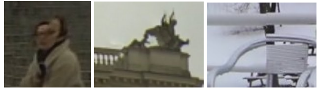
Fig. 1. Examples of parallax errors in panoramic videos. From left to right, the deformation of the person’s head, the misalignment at the top of the building and the ghosting of the statue and the misalignment and loss of part of the chair in the last image. The first is taken from results by [1] which includes a parallax compensation step prior to the final multi-band blending. The second and third are produced using the open source software Hugin [3] with multi-band blending and no parallax compensation.
