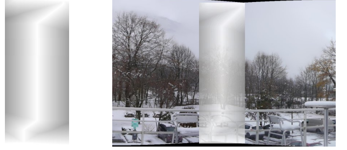
Fig. 3. Example of the suggested mask created around the boundary of the blending line
