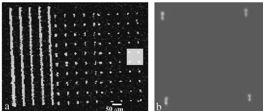
Fig. 5. Fluorescence image of lines and spots obtained from a solution containing fluorescent labels: (a) with a low resolution ScanArrayer™ and (b) with the BioTech BioAnalyser™.
