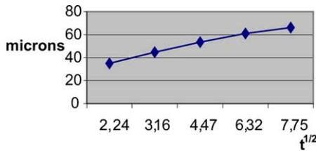
Fig. 7. Spot diameter variation vs. contact time duration.
