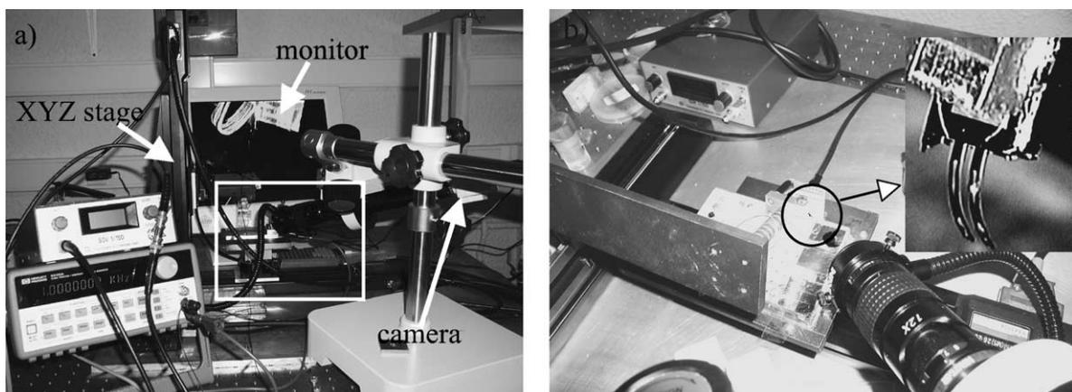
Fig. 3. XYZ motion control system with CCD camera monitoring (a) large view and (b) close-up view.
