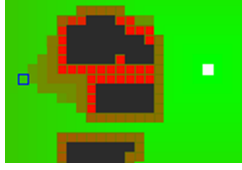
Fig. 1. Illustration of the potential field in the case of obstacle avoidance anticipation. UAV is represented by a dark empty square, the obstacle is represented in dark blue. The cells colored in green are not submitted to any increase. The cells submitted to a potential increase are represented with gradation from brown (smallest) to red (highest).
