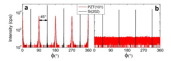
**Figure 2.** XRD φ-scans in the Bragg position of the asymmetrical {h0h} reflections of the {00l}-oriented PZT domains (a) on SRO/STO/Si (sample A) and (b) on Pt/TiO<sub>2</sub>/Si (Sample B).
