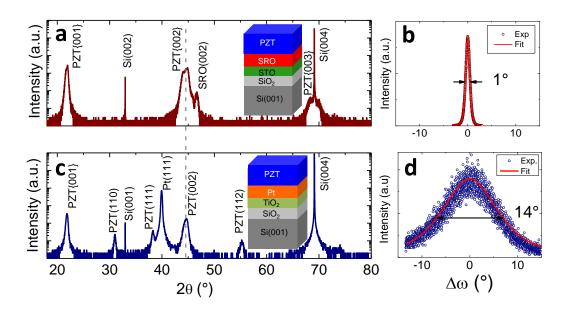
**Figure 1.** XRD  $\theta/2\theta$  scans (a,c) and  $\omega$ -scans around the {002} reflection (b,d) of PZT film deposited on (a,b) on SRO/STO/Si (sample A) and (c,d) on Pt/TiO<sub>2</sub>/Si (sample B).
