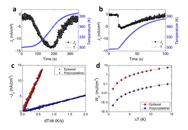
**Figure 4.** (a-b) Pyroelectric current density  $(J_p)$  measured in bottom-top configuration at zero electric field under temperature variations from room temperature to ~400 K, of PZT film deposited on (a) SRO/STO/Si (sample A) and (b) Pt/TiO<sub>2</sub>/Si (sample B). (c)  $J_p$  plotted in function of the heating rate (dT/dt). (d) Density of the pyroelectric energy conversion in function of the temperature variations under 600 kV/cm for both heterostructures.
