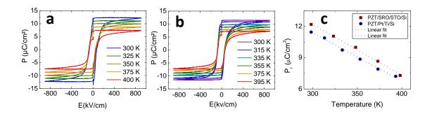
**Figure 3.** Ferroelectric hysteresis loops of polarization measured in bottom-top configuration and PUND method from room temperature to  $\sim$ 400 K of PZT film deposited on (a) SRO/STO/Si (sample A) and (b) Pt/TiO<sub>2</sub>/Si (sample B). (c) Corresponding temperature dependence of remnant polarization ( $P_r$ ).
