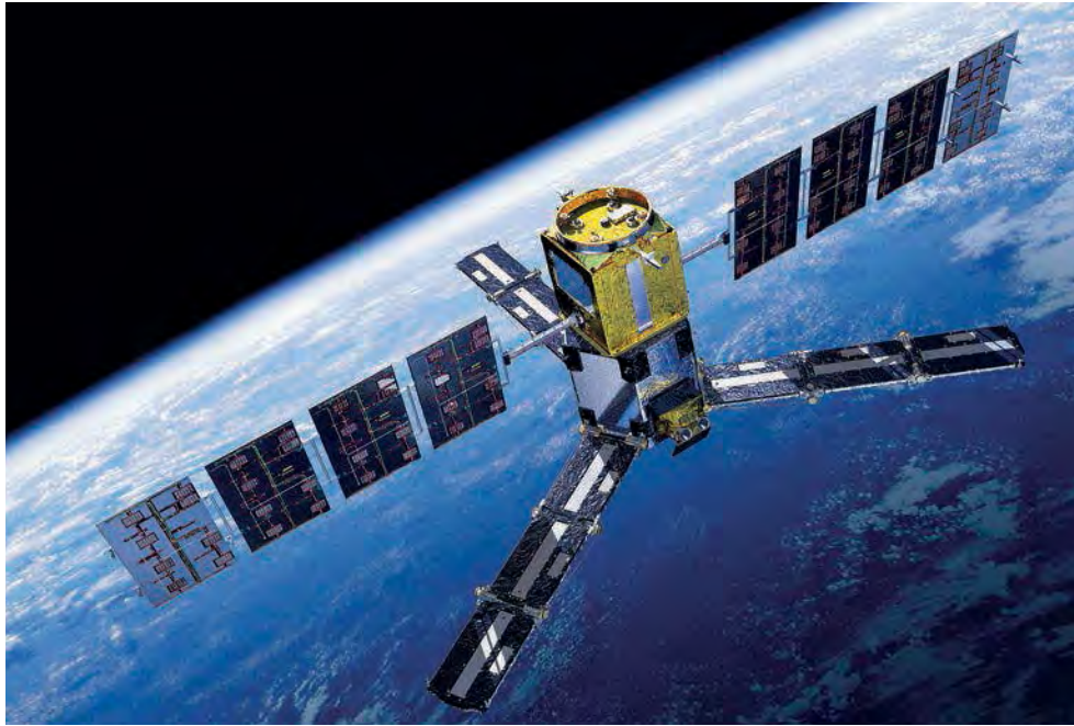
Orbiting SMOS satellite launched on 2 November 2009 by the European Space Agency (ESA). It is the first global climate change observation satellite designed to monitor world marine salinity and soil moisture content.
