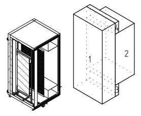
Figure 5: Geometry of the radiation model (right). Correspondence with the inner geometry of the test chamber (left)
