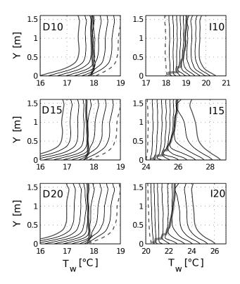
Figure 11: Localization of the fixation temperature  $T_p(y)$  on sequences of wall temperature profiles. The first curve of each sequence is the bold dashed curve, the last curve is the bold full curve. The fixation temperature is located on the thick gray curve
