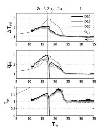
Figure 10: Surface average relative heat flux  $\overline{q}_{rel}''$ , relative temperature difference at the plate  $\overline{\Delta T}_{rel}$ , relative heat transfer coefficient  $\overline{h}_{rel}$ , as a function of the average wall surface temperature  $\overline{T}_w$ . Measurement results from experiments D10, D15, and D20
