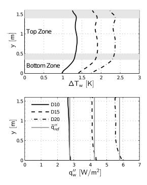
Figure 8: Temperature difference and heat flux profiles during the stationary regime
