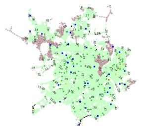
Figure 5. Output of the Algorithm 1 on the Bordeaux Metropolis (France) WDN composed by  $N_V = 60K$  nodes and  $N_E = 66K$  edges. In light green sink nodes that have been saturated, in light red non-saturated sinks. Squares represent sources nodes. Saturated ones are in blue and those with remaining flow are in yellow. The green dot represents sensor nodes saturated during the bidirectional BFS, and the red ones are those where the flow didn't reach the measured flow.
