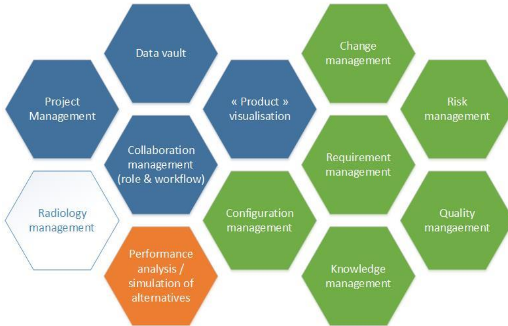
Figure 3: BIM-PLM functionalities elicited for NFD: in green PLM-specific functionalities, in red BIM-specific ones, in blue BIM-PLM common ones and in white NFD-specific one [19]
