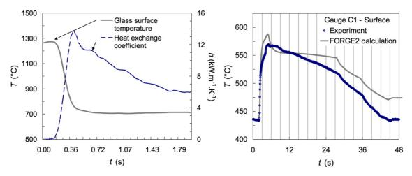
Fig. 11. FORGE2 calculation: boundary conditions during waiting time before pressing (on left hand) and comparison of the surface temperature calculated and estimated by inverse method (on right hand).
