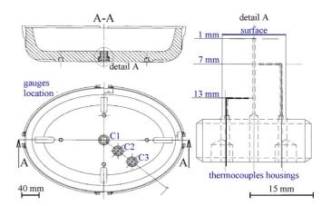
Fig. 3. Description of the instrumented mould: location of the gauges and thermocouples housings.
