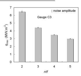
Fig. 5. Influence of the *ntf* parameters from 2 to 5 (max heat flux density and noise).
