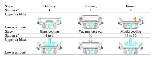
Fig. 1. Different stages of the glass pressing process: upper and lower cooling air flow.
