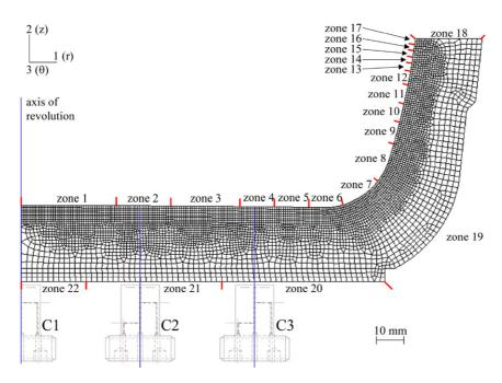
Fig. 9. Meshing of the mould for finite element calculation (Abaqus).
