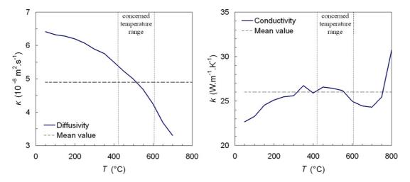
Fig. 6. Evolution of the thermal diffusivity and conductivity of the GX30Cr13 steel with temperature and mean value used for inverse method (Aubert & Duval data).
