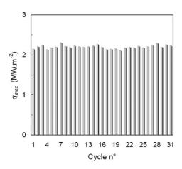
Fig. 7. Successive heat flux density peaks in the production steady state at gauge C1.
