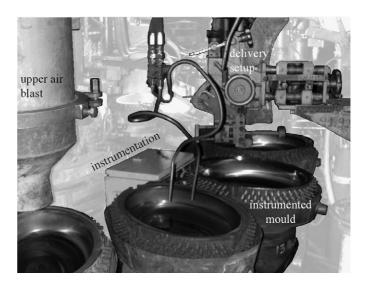
Fig. 2. The instrumented mould in its industrial context just before the delivery.
