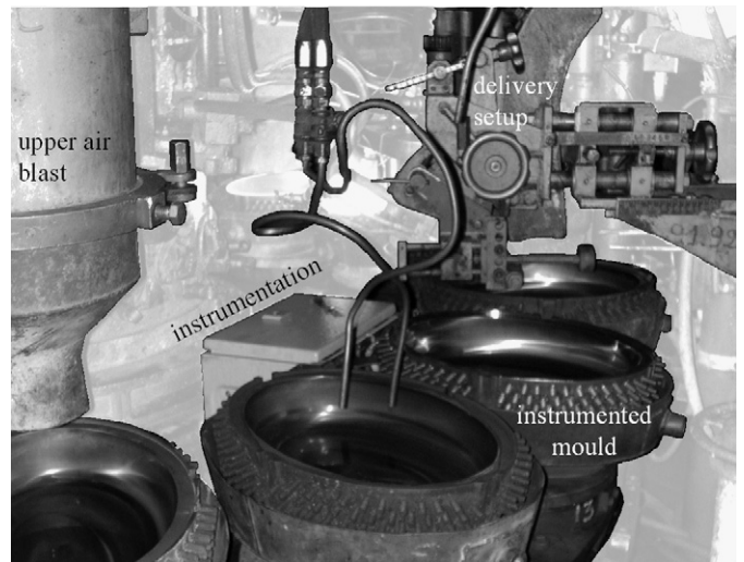
Fig. 2. The instrumented mould in its industrial context just before the delivery.
