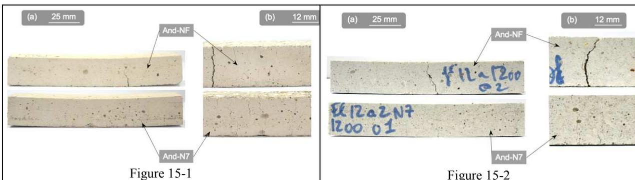
Fig. 15: Macroscopic views of four points bending samples (a: lateral faces, b: zoom on lower faces, in tension) for a non-reinforced grade (And-LCC) and for a Nextel 720<sup>®</sup> reinforced grade (And-N7):
