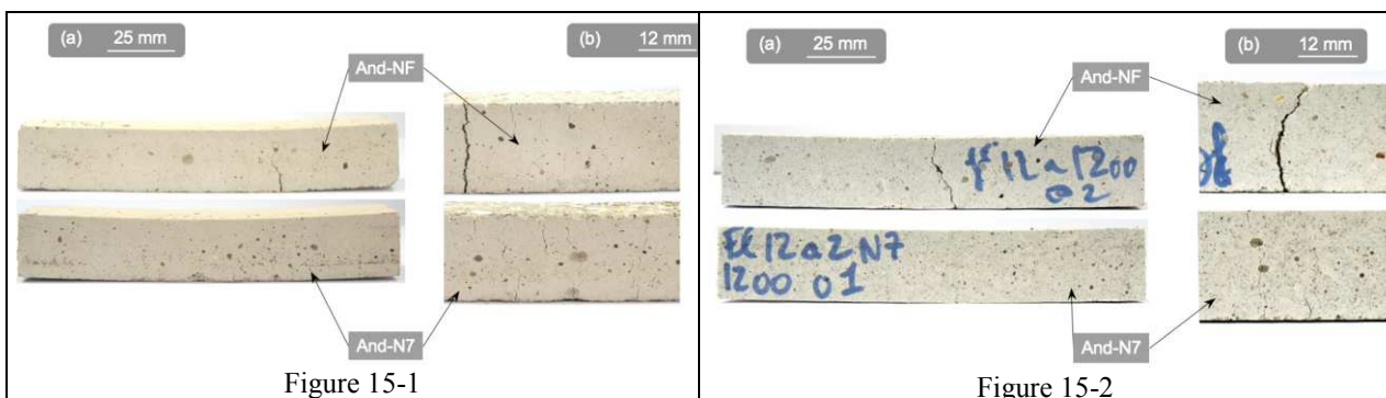
Fig. 15: Macroscopic views of four points bending samples (a: lateral faces, b: zoom on lower faces, in tension) for a non-reinforced grade (And-LCC) and for a Nextel 720 ® reinforced grade (And-N7):
