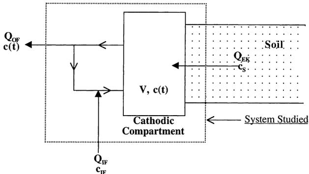
Fig. 6. Cathodic system description for mass balance application.
