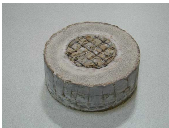
Fig. 7. Photograph of the sample holder and of a brick.
