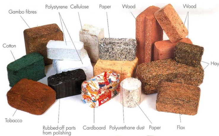
Fig. 1. Some examples of bricks from wood derived and plastic materials (with the agreement of: RUF R Briquetting Machinery).
