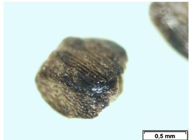
Fig. 15. Wood particle after pyrolysis ( $T = 1223$  K; solid residence time = 0.45 s).
