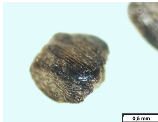
Fig. 15. Wood particle after pyrolysis ( T = 1223 K; solid residence time = 0.45 s).
