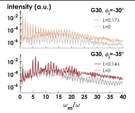
FIG. 5. Intensity profiles of the harmonic spectra integrated over  $82^{\circ} < \phi_{hh} < 87^{\circ}$  for the G30. Colored (gray) lines represent the results of the PIC simulations with (without) the exponential density gradient at the target surface. The preplasma enhances HH generation in both configurations.
