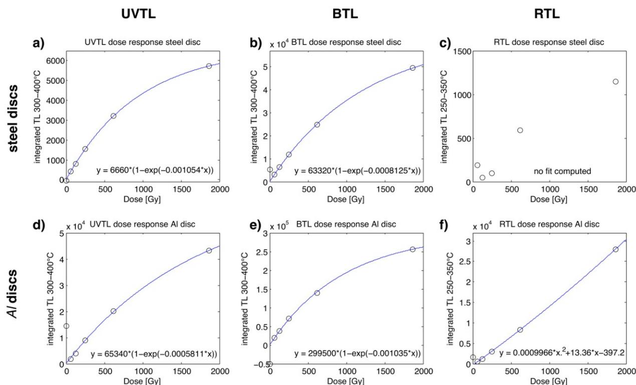
**Figure 3:** TL dose response curves of steel and Al discs for different emissions. The investigated discs are the same as shown in Fig. 1. Integration limits are as indicated on the ordinate. For further details, see text.
