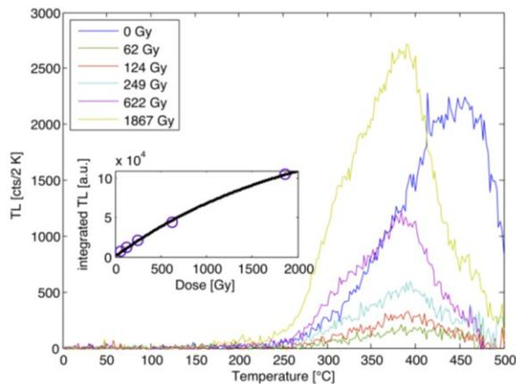
**Figure 6:** Dose response of residual UVTL after blue optical stimulation (470  $\Delta$  30 nm) for 40 s for one Al disc. The inset displays the signal growth for integrated TL (340-440°C) as a function of the regeneration dose, fitted to a single saturating exponential ( $y = a*(1-\exp(-b*x))$ , where  $a = 1.74E+05$ ,  $b = 4.95E-04$  and  $x$  is dose in Gy).
