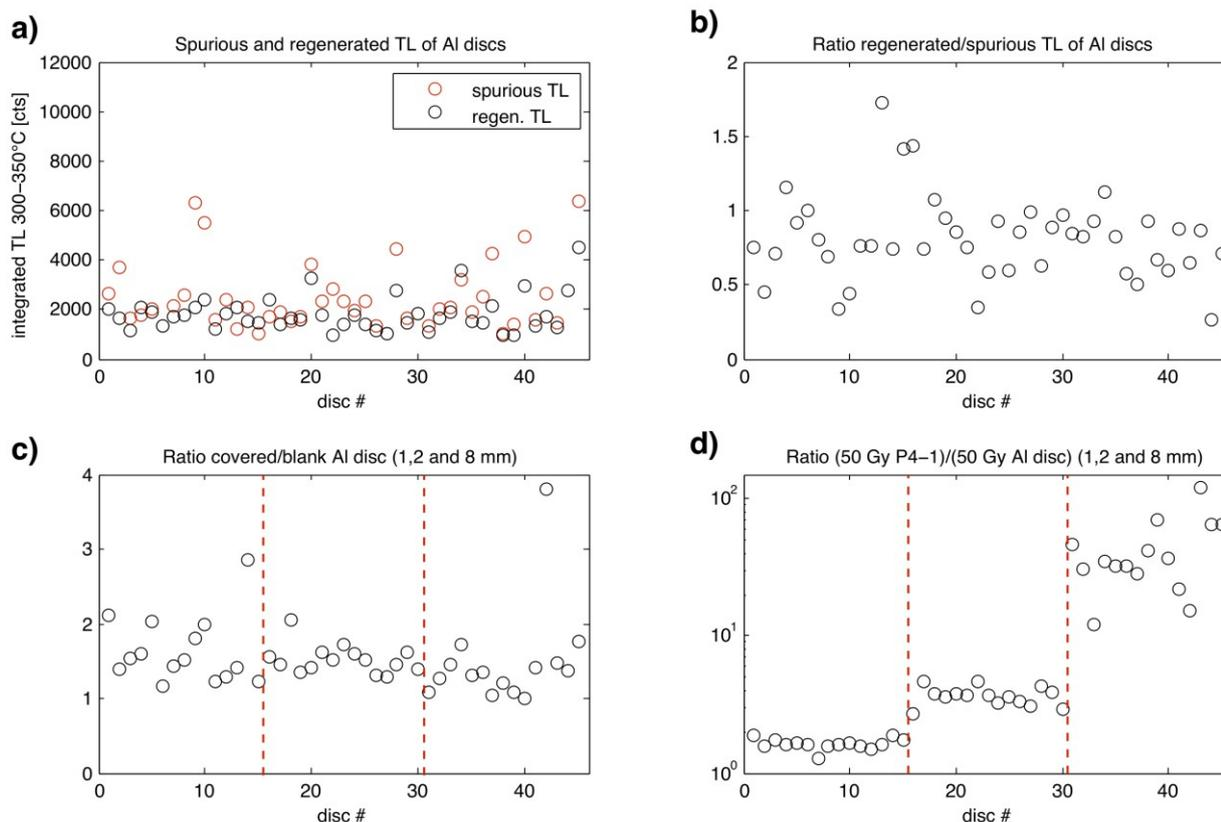
**Figure 2:** Results of the experiment to measure the influence of grain coverage on unwanted signal contributions of used Al discs (UV detection range). Experimental conditions and detailed descriptions are given in the text.
