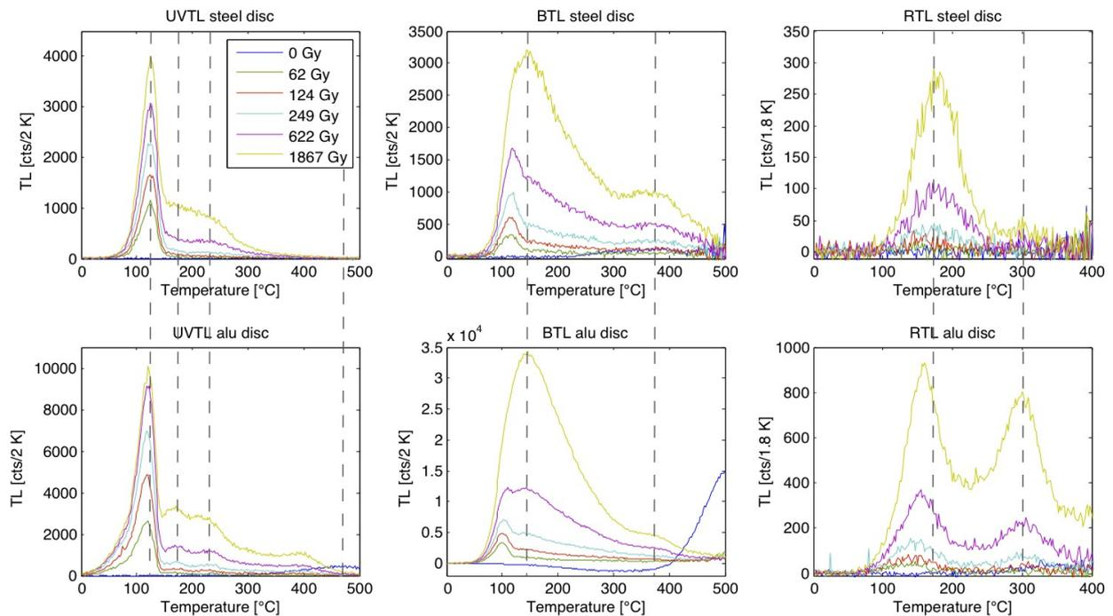
**Figure 1:** Natural and regenerated TL signals from single steel and Al discs for different detection wavelengths. All measurements were performed in Cologne and carried out at  $5 \text{ K s}^{-1}$ . For further details, see text.
