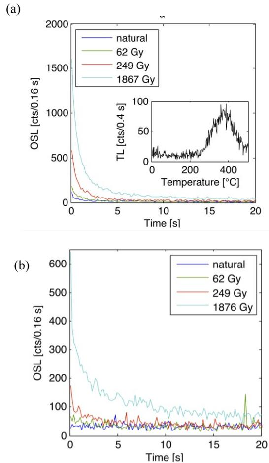
**Figure 5:** Natural (0 Gy) and regenerated OSL signals of single (a) steel and (b) Al discs after preheat (260 °C for 10 s). The inset in (a) shows the residual UVTL measured after  $\beta$ -irradiation of 1867 Gy and 40 s blue optical stimulation (470  $\Delta$  30 nm). For further details, see text.
