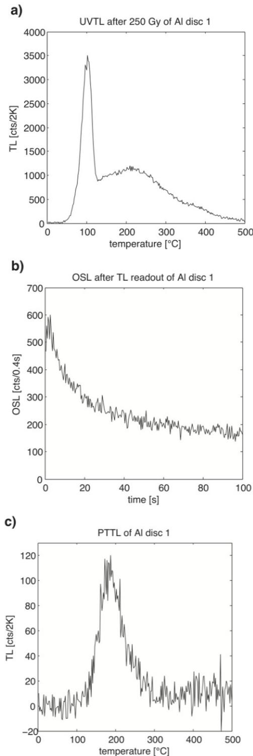
**Figure 7:** PTTL measurement in the UV of an Al disc after a  $\beta$ -dose of 250 Gy was given: a) background subtracted TL measurement up to 500 °C after irradiation, b) subsequently recorded blue stimulated OSL signal, c) photo-transferred TL signal after optical signal depletion.
