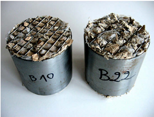
Fig. 6. Photograph of the bricks composed of cardboard and polyethylene ground elements.
