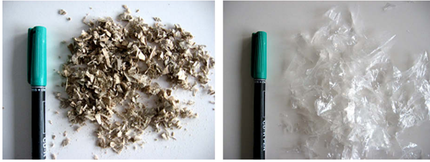
Fig. 5. Photographs of the ground elements of cardboard and of polyethylene. The length of the cap on the pen is 42 mm.
