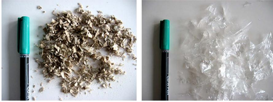
**Fig. 5.** Photographs of the ground elements of cardboard and of polyethylene. The length of the cap on the pen is 42 mm.
