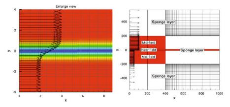
Fig. 2 Mixing layer acoustic pressure field. Initial condition (*left*) and computational domain with sponge layer (*right*)
