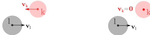
Figure 10: Two motion scenarios, both having the same category, i.e., S_{14}(DC_-) , in the motion representation Motion-RCC. The fact that in the second scenario the entity k is motionless is not a hindrance for a scenario categorisation.
