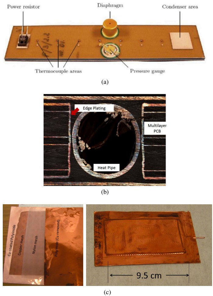
Fig. 4: Dual-phase passive cooling systems using PCB technology: (a) a heatpipe formed by a cavity in a PCB [53]; (b) a 2 mm diameter tubular heatpipe inserted in a PCB (cross section view) [54]; (c) a thermal ground plane (vapor chamber) which can be inserted in a PCB stack-up.
