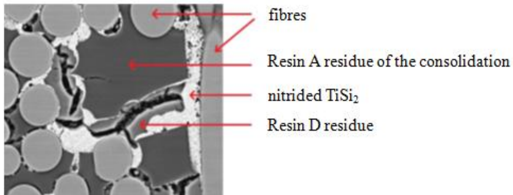
Figure 4. SEM micrograph of polished cross section of a composite (2D Nicalon preform) elaborated with one impregnation of TiSi_2 powder, nitrided 5 h at 1100^\circ C and with one PIP cycle using (CMC2).
