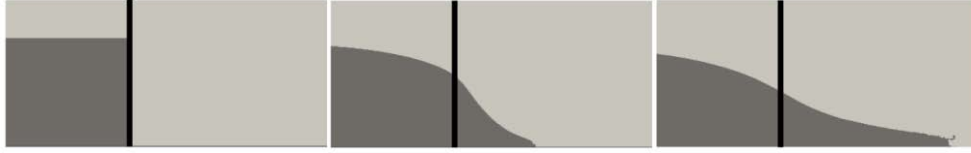
Figure 2. Dam-break on dry bed. Screen capture taken at T=0 , T=0.88 , and T=1.57 (these simulations are in good agreement with experimental results given in figure 3 of [7]).
