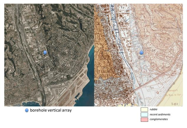
Figure 2. The future Nice borehole test site: satellite image on the left side and geological map on the right side
