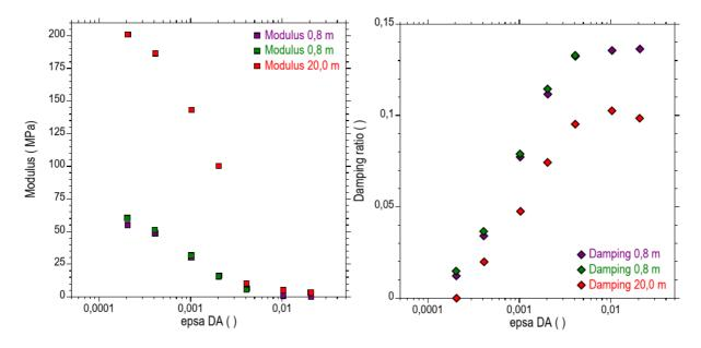
Figure 6. Left: Relationships between secant modulus and shear strain –Right: Relationships between hysteretic damping ratio and shear strain
