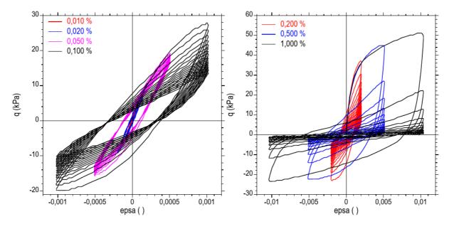
Figure 5. Relationships between deviatoric stress q and shear strain epsa – Several successive sequences of undrained cycles in a range of axial deformation: 0,010 % - 0,020 % - 0,050 % - 0,100 % - 0,200 % - 0,50 % -
