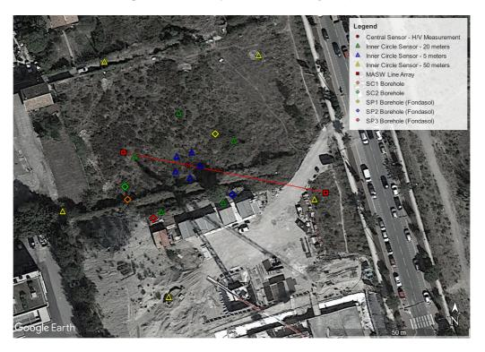
Figure 7. Position of the stations of the seismic array (triangles) and the MASW profile. Boreholes SC1 and SC2, where accelerometers will be installed, are shown by orange and green diamonds. Geotechnical boreholes SP1, SP2 and SP3 by yellow, blue and red diamonds
