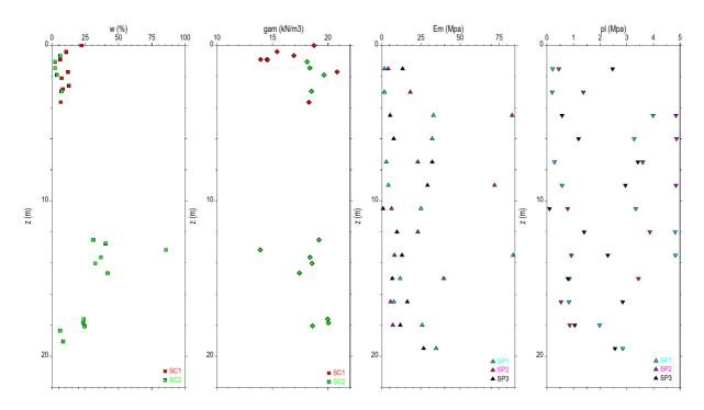
Figure 4. From left to right: Water content, unit weight, pressiometric modulus and net limit pressure versus depth
