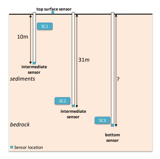
Figure 10. Scheme of the future installation
