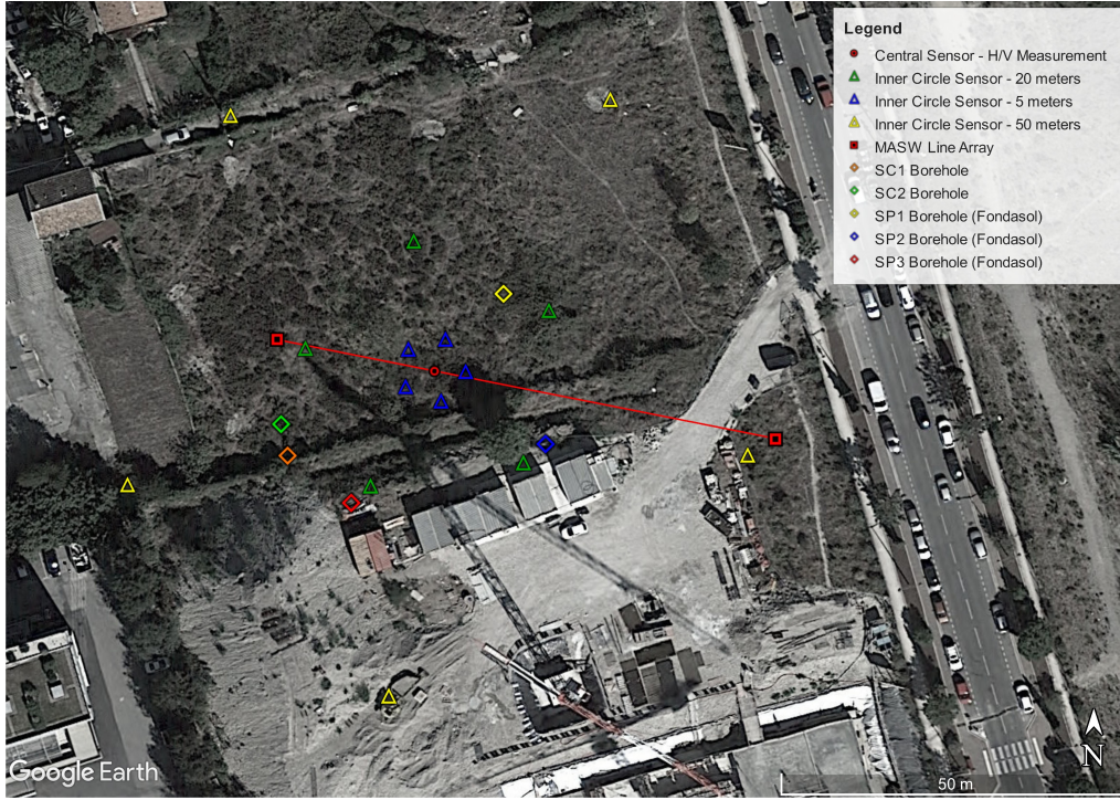
Figure 7. Position of the stations of the seismic array (triangles) and the MASW profile. Boreholes SC1 and SC2, where accelerometers will be installed, are shown by orange and green diamonds. Geotechnical boreholes SP1, SP2 and SP3 by yellow, blue and red diamonds
