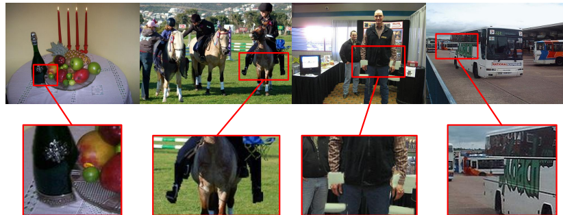
Fig. 6. Illustration of artifacts arising from enlargement augmentation. In the enlargement data augmentation, an instance is cut out of the image, up-scaled by a small factor and placed back at the same location. This approach leads to blending artefacts. Modified images are given in the top row. Zoomed parts of the images centered on blending artifacts are presented in the bottom line.
