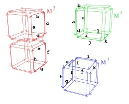
**Figure 5.** A 3-dmap DM that represents the 3-map of Figure 1b which has been decomposed into 3 blocks  $M^1$ ,  $M^2$ ,  $M^3$ . Critical darts are labeled with lowercase letters  $a, \ldots, 1$ , and are drawn in bold.
