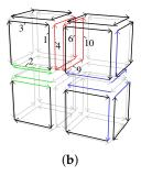
**Figure 1.** (a) A 3D mesh composed of 4 cubes,  $V_0$ ,  $V_1$ ,  $V_2$ ,  $V_3$ , two by two adjacent; (b) The corresponding 3-map having 96 darts (24 for each cube) where some darts are numbered.
