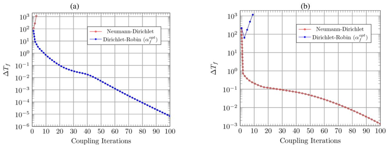
Fig. 3: Convergence vs coupling iterations. (a) Weak thermal interaction ( $\lambda_s = 10.0 \text{ Wm}^{-1}\text{K}^{-1}$ ,  $Bi_v = 0.47$ ). (b) Strong thermal interaction ( $\lambda_s = 0.01 \text{ Wm}^{-1}\text{K}^{-1}$ ,  $Bi_v = 462.5$ ) [9].
