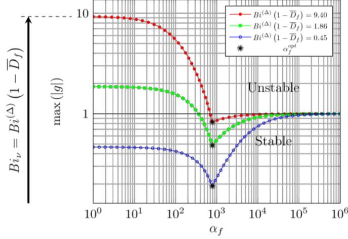
Fig. 1: Temporal amplification factor ( $\max|g|$ ) and optimal coefficient for three different intensity values of the fluid-structure interaction  $Bi_v$  in the case of Dirichlet-Robin interface procedure [9].
