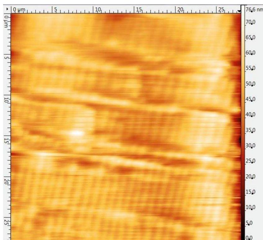
**Figure 6.** Atomic force microscope picture ( $28 \times 28 \mu\text{m}$ ) of a polymerized 8CB thick film with 7 wt % of monomers. The sample was observed more than one year after its preparation, revealing a well-defined undulation of a period  $\sim 1 \mu\text{m}$ , consistent with the optical microscopy results. The topography scale is shown on the right-hand side of the image.
