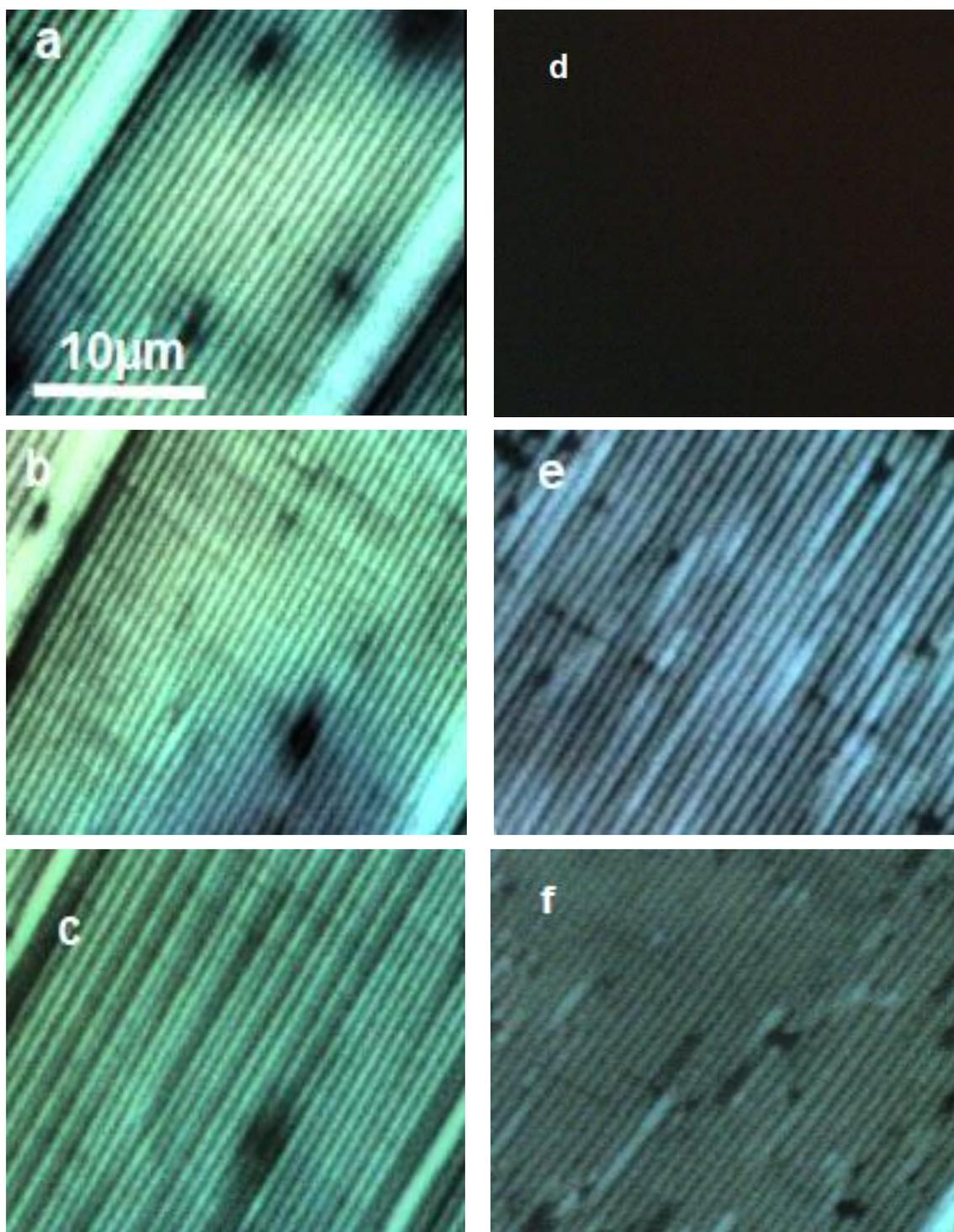
**Figure 7.** Crossed polarizer images of the 10 wt % irradiated thin film (a) in the Sm-A phase at 23 °C; (b) in the nematic phase at 27 °C and (c) 29 °C; and (d) in the isotropic phase at 42 °C; (e) on re-cooling at 23.5 °C; after heating at 70 °C (f) and at 45 °C.
