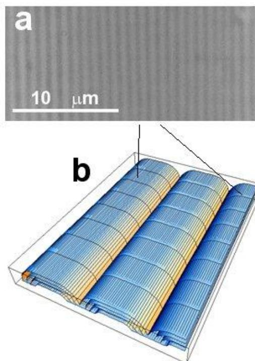
**Figure 1.** (a) Polarized reflection image of oily streaks in the smectic-A (Sm-A) phase of 8CB. Scale bar is parallel to the easy axis of the substrate's alignment layer; (b) Schematic representation of oily streaks.
