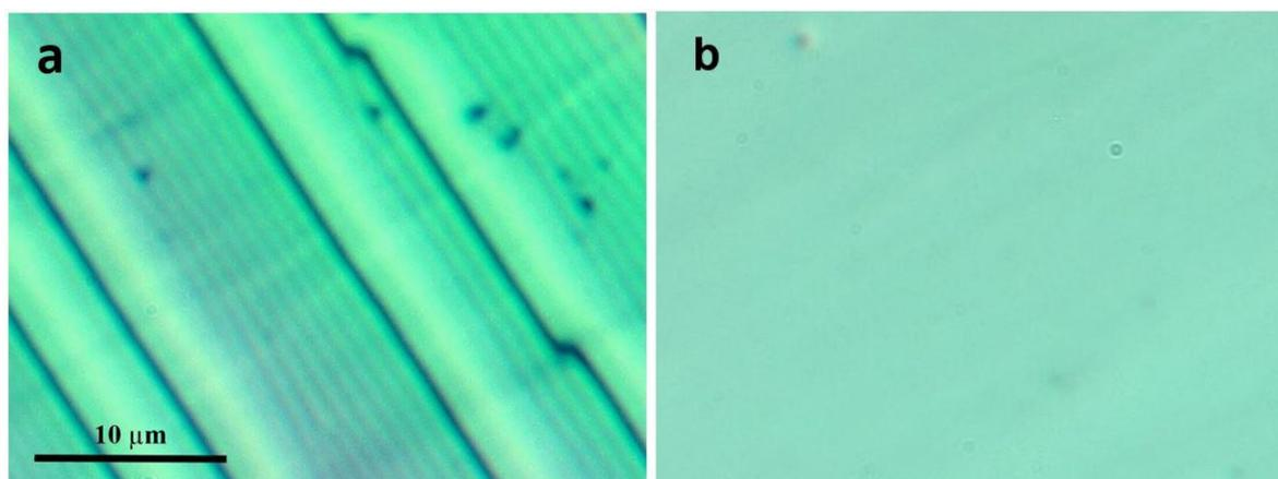
**Figure 2.** Crossed polarizer images of the irradiated 3 wt % thick film in the Sm-A phase at 29.5 °C (a) and in the nematic phase at 31 °C (b). In 2a, light striations can be seen running from the lower left to the upper right, which are due to inhomogeneities in the substrate rubbing. Scale bar represents 10 μm.
