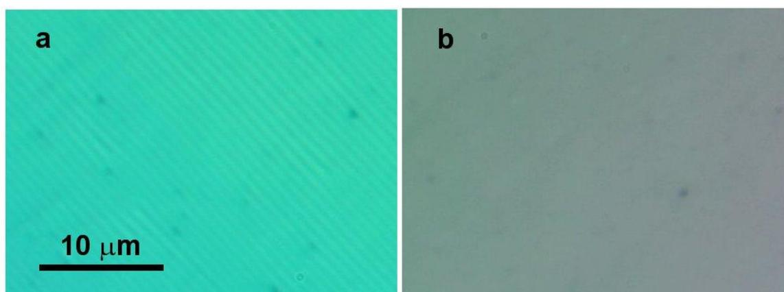
**Figure 3.** Crossed polarizer images of (a) the non-irradiated 10 wt % thick film in the Sm-A phase at 22.6 °C and (b) in the nematic phase at 25 °C. Notice in (a) the oily streaks. Scale bar represents 10 μm.
