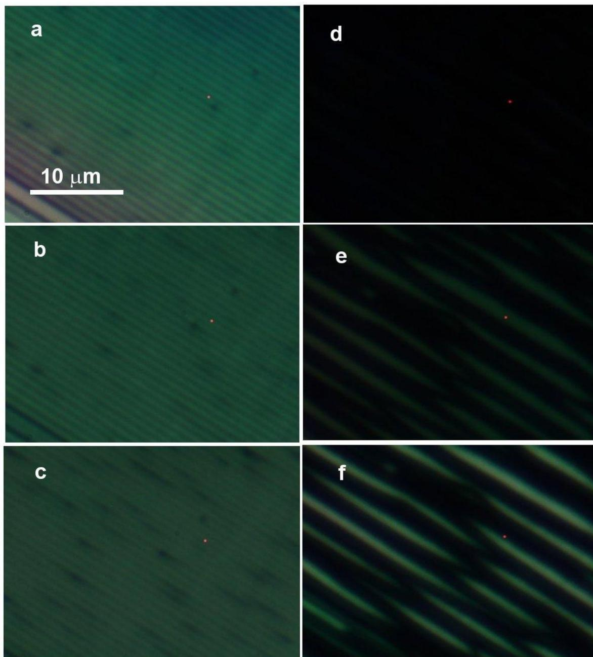
**Figure 5.** Crossed polarizer images of the 10 wt % irradiated thick film (a) in the Sm-A phase at 23 °C; (b) in the nematic phase at 27 °C and (c) 29 °C; and (d) in the isotropic phase at 42 °C, and then on re-cooling at (e) 38 °C and (f) 23.5 °C.
