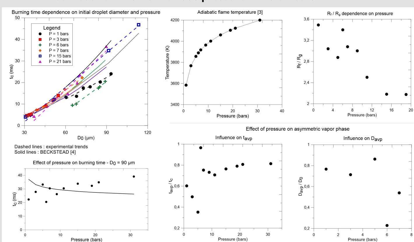
Varying pressure in a low range seems to modify related parameters of asymmetric vapor phase. Influence of higher pressure is then less considerable.
