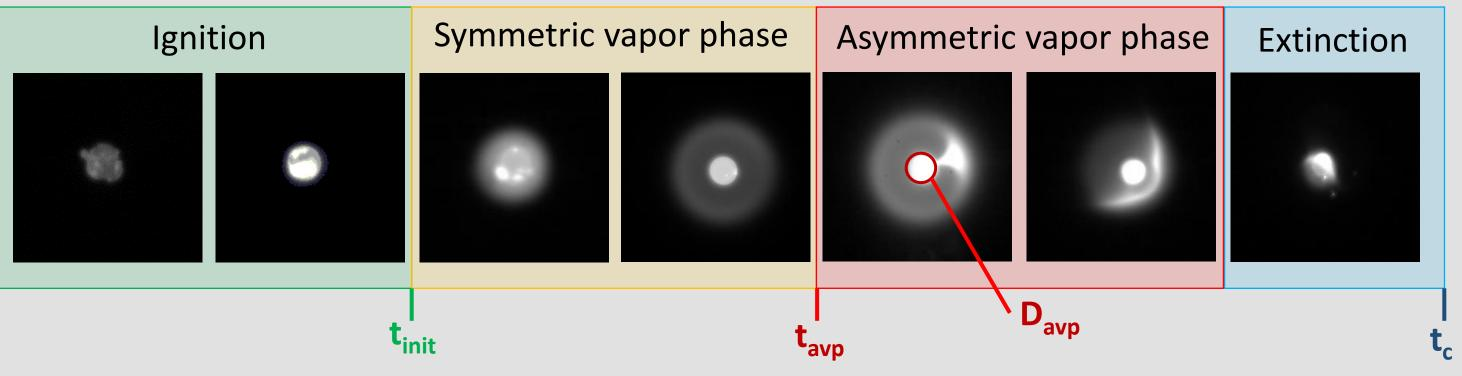
Existence of a symmetric and asymmetric vapor phase (avp) regimes  $\succ$  Introduction of related parameters :  $\mathbf{t}_{avp}$  and  $\mathbf{D}_{avp}$ , respectively time and droplet diameter before asymmetric phase occurrence.
