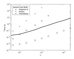
Fig. 3. Computational time of the proposed Frank-Wolfe algorithm, Newton's method [7], FrameSense [8] and weighted least-squares [25], in function of the size of the discretization L, with m=20, for gaussian matrices.
