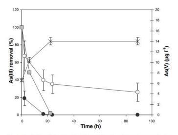
Fig. 1. Evolution of dissolved As(III) as a function of time in groundwater inoculated with sterilized (open circle) and unsterilized (full circle) biofilm or pure bacterial strain B2 (grey square) and the corresponding As(V) concentration in the experiment with isolated strain B2 (cross). Original As(III) concentration in groundwater was  $6.4 \ \mu g \ l^{-1}$ , pH 7.4,  $T = 30 \ ^{\circ}$ C. The error bar corresponds to the standard deviation obtained for four replicates.
