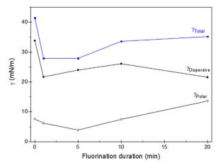
**Fig. 3.** Change in the surface energy ( $\blacksquare$ ) of silver fir as a function of the fluorination duration; the dispersive ( $\bullet$ ) and polar ( $\times$ ) components are also reported.
