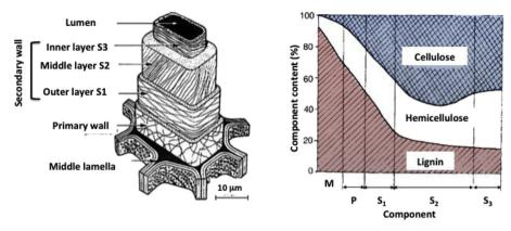
Fig. 4. Components' relative content and microstructure of wood [32,33].
