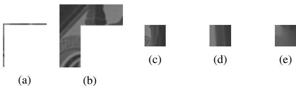
Fig. 9: Prediction of a block of size 16 \times 16 pixels via the best H.265 mode in terms of PSNR and PNNS: (a) H.265 causal neighborhood, (b) PNNS context, (c) block to be predicted, (d) predicted block via the best H.265 mode (of index 25) in terms of PSNR, and (e) predicted block via PNNS.
