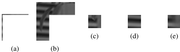
Fig. 8: Prediction of a block of size 16 \times 16 pixels via the best H.265 mode in terms of PSNR and PNNS: (a) H.265 causal neighborhood, (b) PNNS context, (c) block to be predicted, (d) predicted block via the best H.265 mode (of index 11) in terms of PSNR, and (e) predicted block via PNNS.
