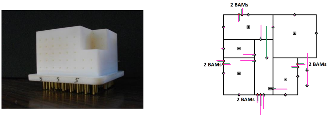
Figure 11: Scale model (left) and CONTAM simulation of natural ventilation through the BAM (right).
