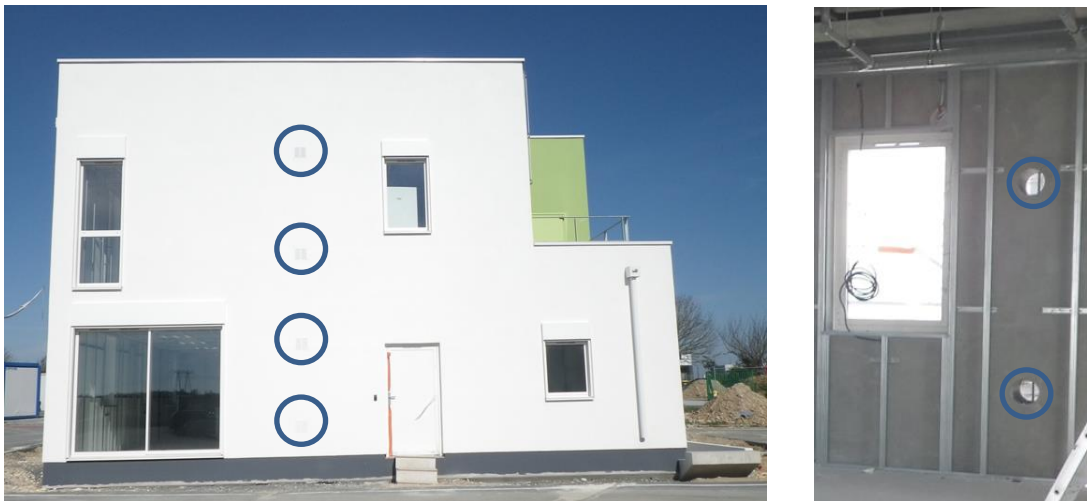
Figure 2: BAM locations in the test house (left: outside view; right: inside view).
