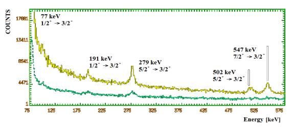
**Figure 2.** The total spectrum recorded by ORGAM detectors, upper curve, compared with the spectrum relative to the central part of the mass-TKE distribution, lower. The <sup>197</sup>Au transitions identified in the total spectrum are marked with their energy and angular momentum.
