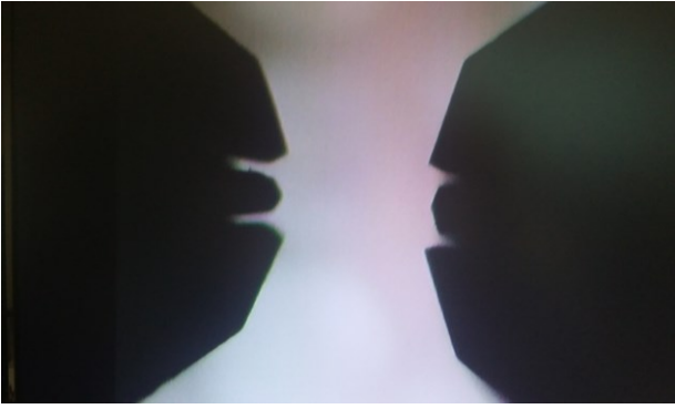
Fig 5: Image of the Picoprobe 50 \mu\text{m} pitch with waveguide used in G-band (140 GHz–220 GHz) measurement. Note that two other Picoprobes are also used in measurement but their images are not shown.
