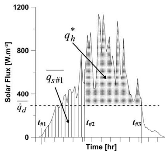
Figure 5: Graphical representation of the operation of a solar-powered chiller. Between  $t_{\#1}$  and  $t_{\#2}$ , solar heat is stored into the solar loop for preparing operation (hatched surface); the chiller is switched-off. Between  $t_{\#2}$  and  $t_{\#3}$ , only the part of insolation lying over the dissipation rate is transferred to the chiller (grey surface).
