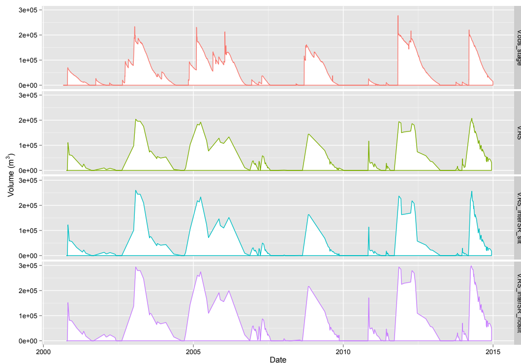
Figure 11. Daily volumes for Gouazine lake over 2000–2014 based on: (i) observed stage data; (ii) Landsat data using a site-specific rating curve; (iii) Landsat data using the power relation adapted for silting; (iv) Landsat data using the power relation not adapted for silting.
