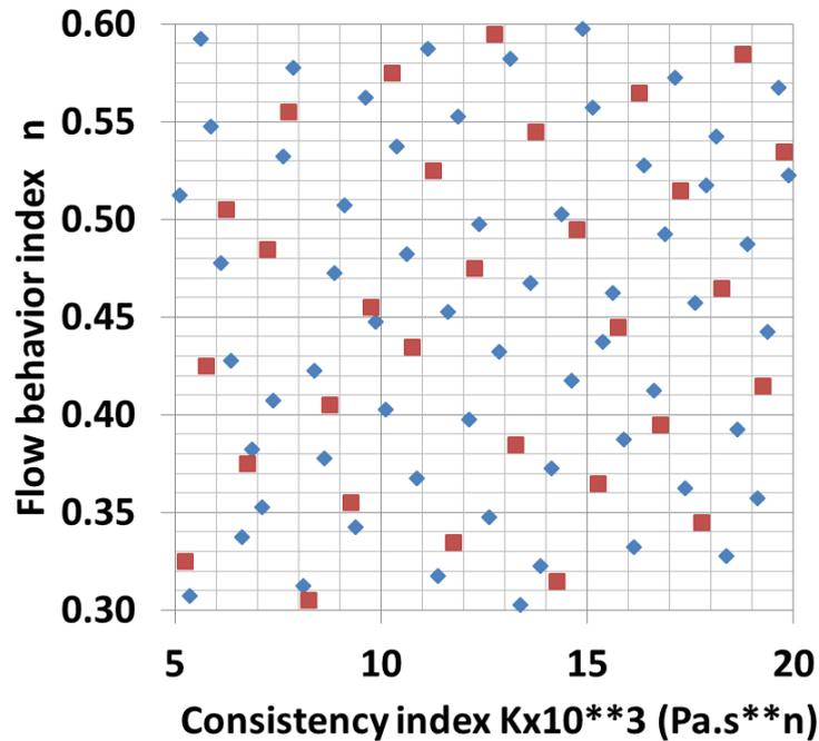
Figure 5: Sets of  $(K, n)$  couples generated by Improved Hypercube Sampling. The set of blue diamond dots is used as input data for ROMs identification. The set of red square dots is used as input data for ROMs validation.
