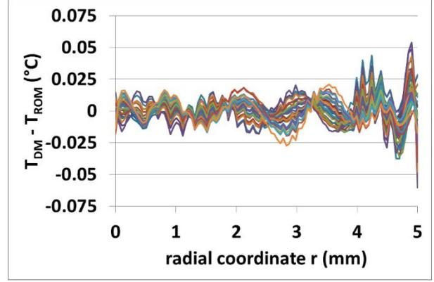
Figure 13: ROMs validation. Difference between outlet temperature profiles computed by DM and order 5 ROM for 30  $(K, n)$  couples.
