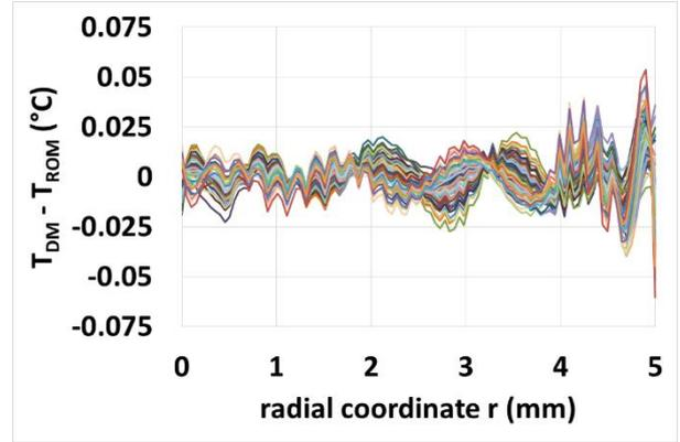
Figure 9: ROMs identification. Difference between outlet temperature profiles computed by DM and order 5 ROM for 60  $(K, n)$  couples.
