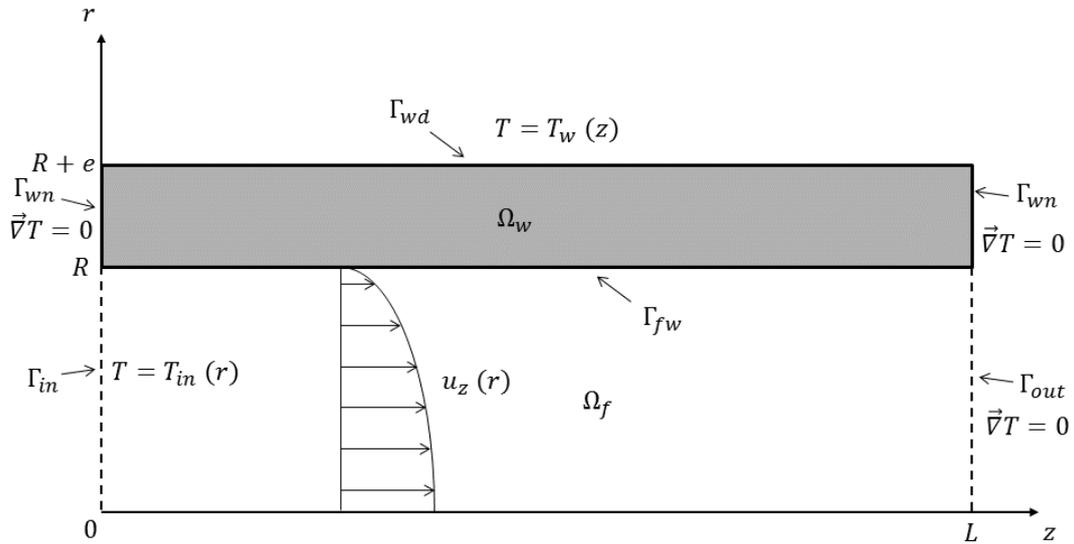
Figure 2 : Flow in circular channel. Schematic view including boundary conditions
