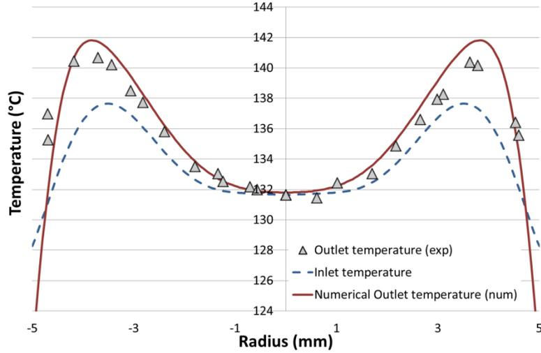
Figure 4: Comparison of experimental and numerical outlet temperature profiles of an elastomer flow. The inlet temperature profile is drawn in dashed line.
