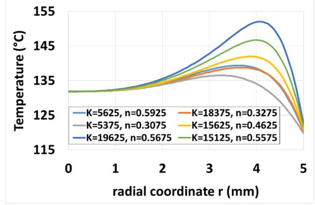
Figure 7: Outlet temperature profile computed by DM for 6  $(K, n)$  couples among the 60 used for ROMs identification.
