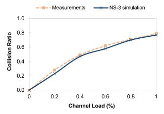
Fig. 4: Comparison between measured and simulated values: collision ratio in function of the channel load.
