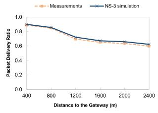
Fig. 3: Comparison between measured and simulated values: packet delivery ratio in function of the distance between end devices and the gateway.
