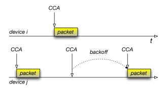
Fig. 6: Principle of CSMA: device j sends a packet after a CCA and backs off when channel is busy.
