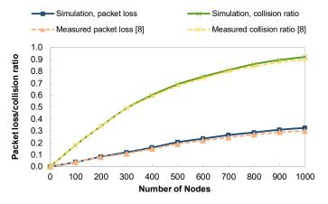
Fig. 5: Comparison between simulated values and measurements by Haxhibeqiri et al. [8] showing the impact of the capture effect.
