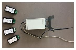
Fig. 1: The LoRa testbed with 4 Semtech SX1272LM1BAP end devices and a Kerlink IoT gateway.
