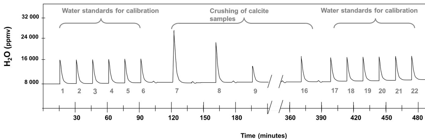
Figure 3: Schematic of water vapour evolution over the course of a regular analysing day. Peaks 1 to 6, are 0.3  $\mu\text{L}$  injections of water standards for calibration MAZA (1, 2), -5‰ (3, 4), and -8‰ (5, 6). Peaks 7 to 16 corresponds to the released fluid inclusion water after calcite crushing. Peaks 17 to 22, are 0.3  $\mu\text{L}$  injections of water standards for calibration MAZA (17, 18), -5‰ (19, 20), and -8‰ (21, 22).
