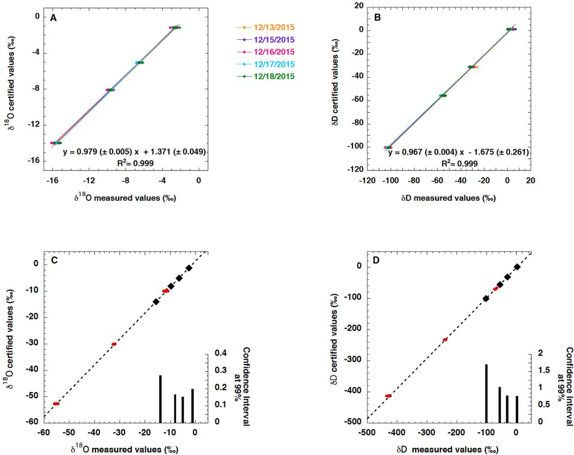
Figure 6: A. and B. Values of four 0.5  $\mu\text{L}$  injections of laboratory standard (-5‰, -8‰, ESKA, and MAZA) over different days. The averaged calibration equation is represented in each plot. C. and D. Mean values for the calibration and confidence interval at 99 % for each point of calibration. The red dots are other laboratory standards (DOMEC; NAN; -10 ‰; -30 ‰; Table 1) analyzed to test the validity of the calibration for out of range water standards.
