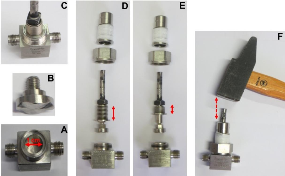
Figure 2: Different sections of the crushing device: A. The modified vacuum valve body milled to obtain a 1 cm diameter cavity, B. The modified valve stern cap used as a power hammer, C. The valve body and valve stem are sealed with airtight metallic-metallic connexion using metallic washer, D. and E. present the valve bellow before (D) and after (E) the crush, F. Picture presenting the vertical movement of the hammer hammering the top of the valve stem.
