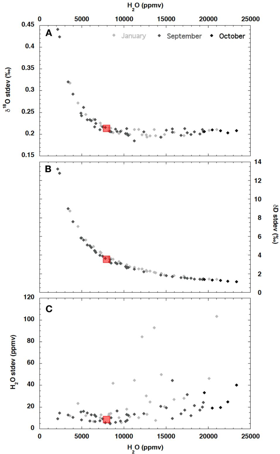
Figure 4: Water background stability. Each point corresponds to the standard deviation of A.  $\delta^{18}O$ , B.  $\delta D$ , and C. the water concentration ( $H_2O$ ). Each set background was analyzed over a period of three hours and we averaged the data over the last 30 minutes. Red squares correspond to the background values chosen.
