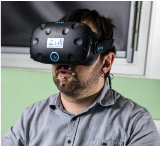
Figure 1: Beaming the head, eyes, lips and hands of Nina, the GIPSA-Lab iCub robot. Left, we retarget the head, eyes, lips and hand movements of the pilot to directly control the corresponding segments of Nina; The pilot receives audiovisual feedback from Nina’s eye-embedded cameras and ear-microphones in the head-mounted display. Right: the remote HRI scene, where Nina instructs subjects to move objects. © Cyril FRESILLON / GIPSA-lab / CNRS Photothèque
