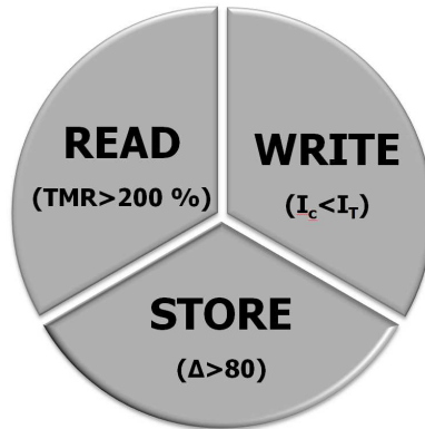
Figure 14. An example STT-MRAM Trilemma. Simultaneously three properties have to be satisfied: reading, writing and storing. In this example is necessary to have TMR > 200\% for reliable reading, switching current less than that supplied by a small transistor for small cell size, and thermal stability factor \Delta > 80 to meet a desired data retention goal.
