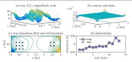
**Fig. 6** Setup of the groundwater inversion example. (a) "True" transmissivity field. (b) Sources and sinks. (c) Drawdown field resulting from the true transmissivity field, with observation wells indicated by black dots. (d) Data y; circles represent the noise-free drawdowns at each well, while crosses represent the observed drawdowns with measurement noise.
