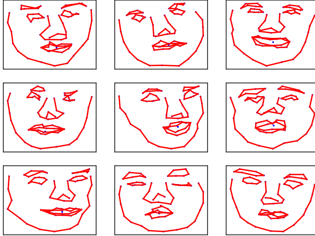
Figure 3: Shapes generated using perturbation of 50% of the landmarks with maximum magnitude of 5% of the shape size.
