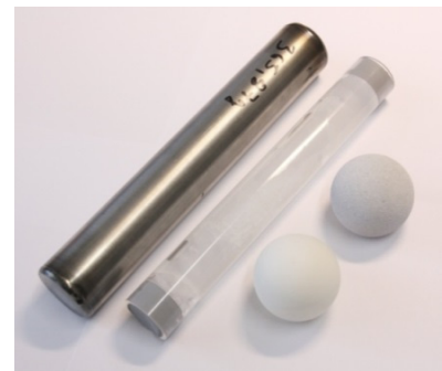
Fig. 22: Macroscopic encapsulated PCM for mobile latent thermal energy storage of University of Bayreuth
